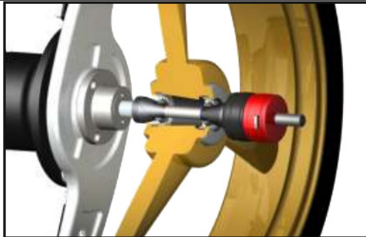
Shaft with centering cones.
